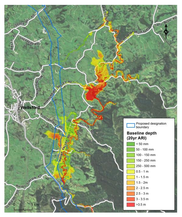
Figure 17 - Modelled flood extents and depths for the Hōteo River for existing conditions for floods of 20 year ARI
