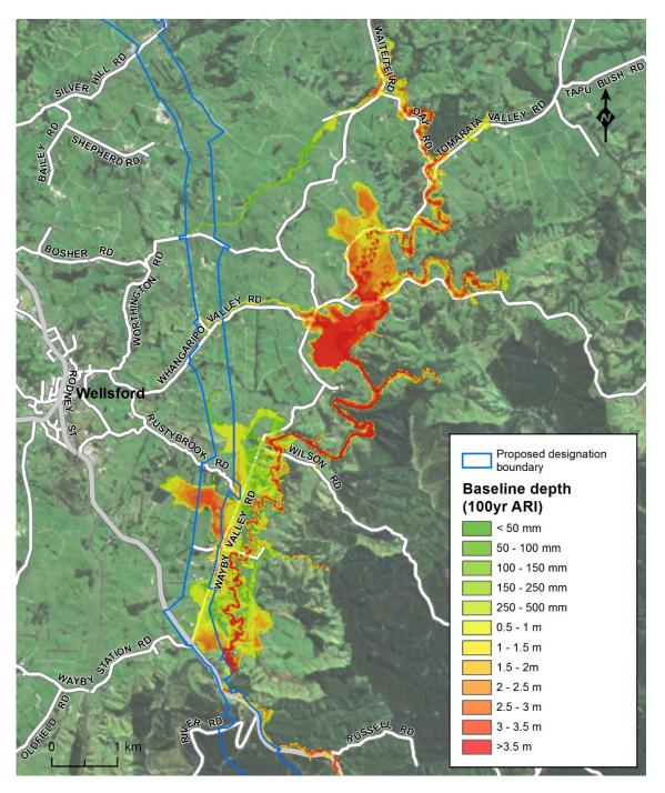
Figure 16 - Modelled flood extents and depths for the Hōteo River crossing for existing conditions for floods of 100 year ARI
